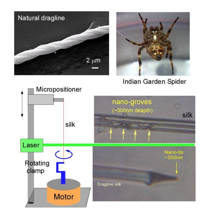
*Figure 1*: A picture of the spider and electron microscope image of its twisted silk. The experimental setup is schematically shown in the bottom left. Bottom right shows some nanoprocessed silk using femtosecond laser pulses.
