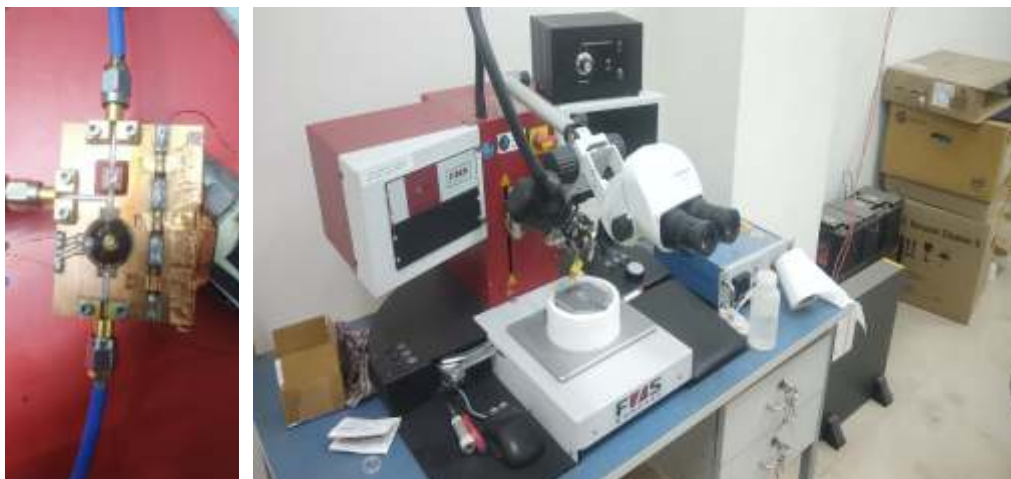
On the left a Device made with PCB Prototyping system. On the right an Ultrasonic wire-Bonder used to make fine connections
