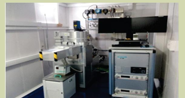
Figure (a) The gas distribution system for the Plasma etch system (b) The actual plasma etch system in the class 10,000 cleanroom.
